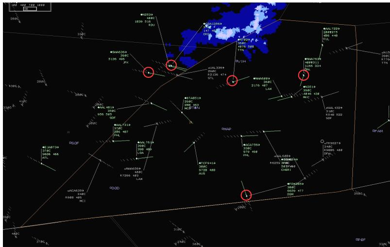
Figure 1. A sample screen-shot obtained from the aircraft-based complexity assessment. A controller evaluated all the aircraft under jurisdiction. Aircraft contributing high complexity were identified in red circles.
