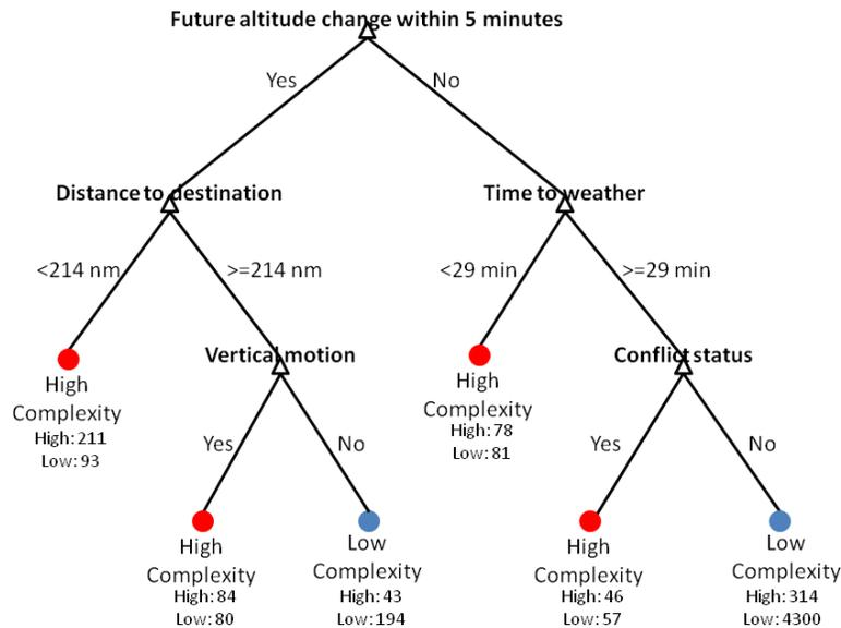
Figure 4. Classification tree trained with 18 observable states. The numbers under each node are the counts of true high complexity aircraft and the true low complexity aircraft for the whole data set including training data and test data.
